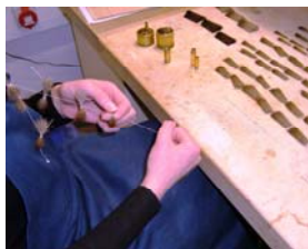
A da Vinci brushmaker hand-making sable brushes at their factory in Nuremberg.
